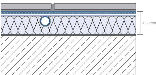
Cross-section: conventional underfloor heating installation height from approx. 85 mm
