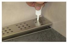
**1** The grate cover is raised and lifted out using the grate lifter (white plastic lever) included in the scope of delivery.
